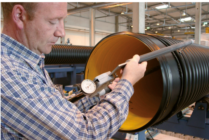
Checking of the wall thickness
