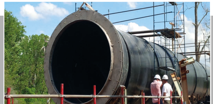
DN/OD 4000 mm solid wall pipe with SDR 11
