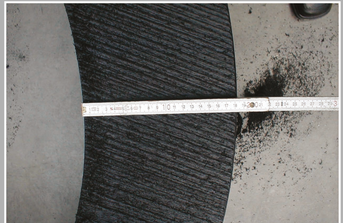
Solid wall polyethylen pipe, s = 180\text{mm}
