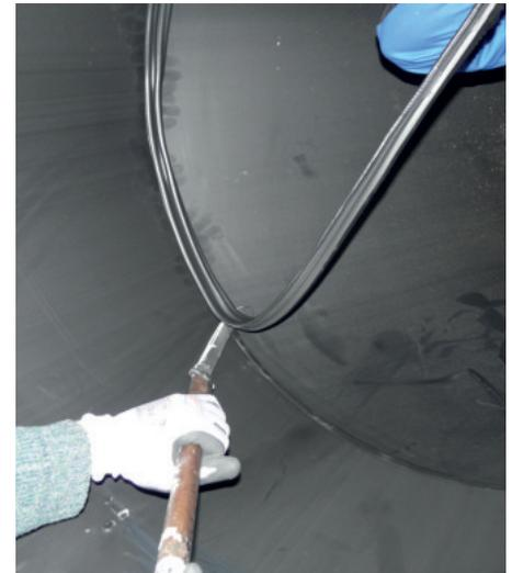
Fig. 6 - Inner bead removal
